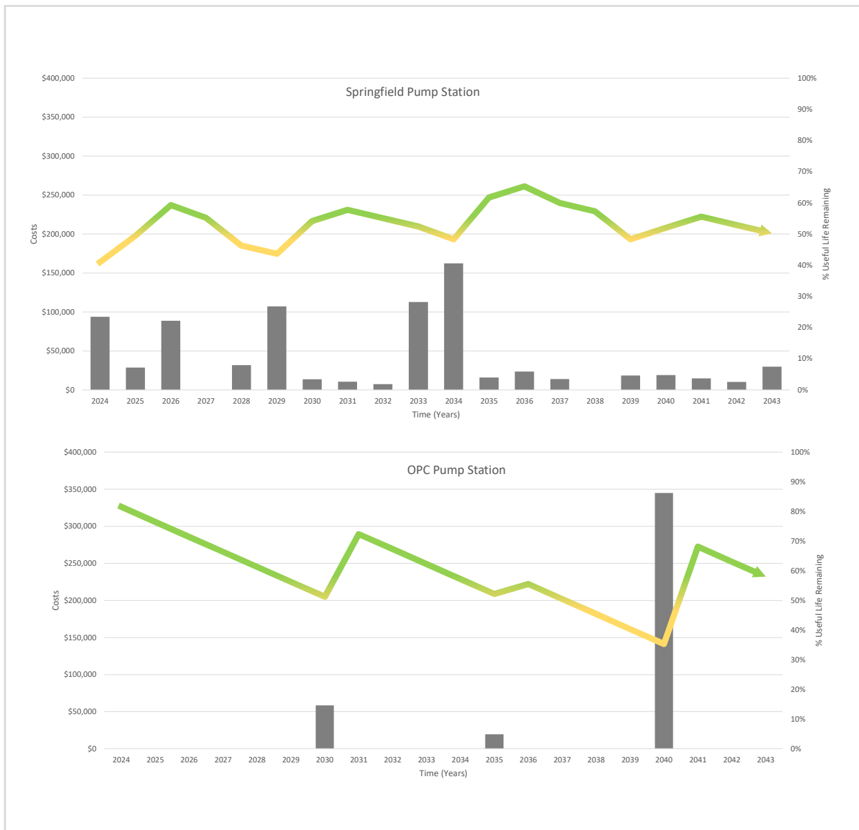
Figure 14 Condition Forecast – Pump Stations
