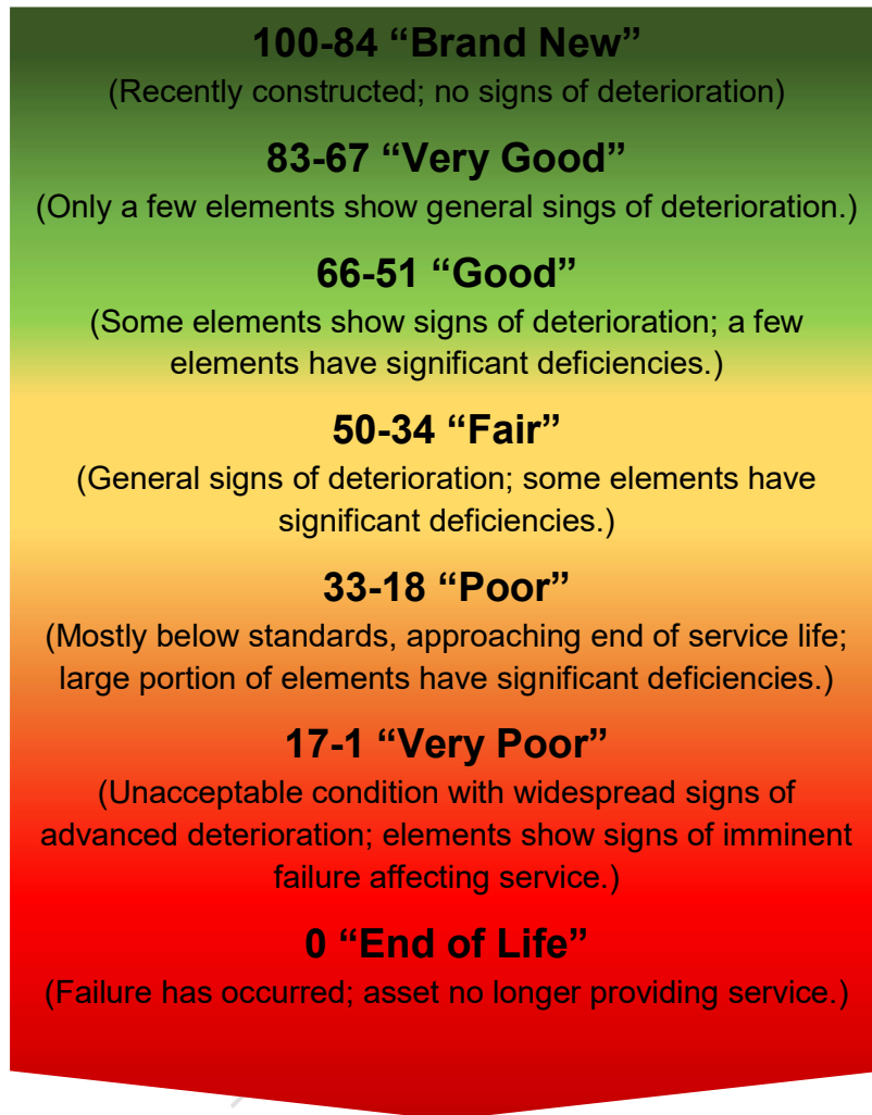
Figure 7-1 Condition States Defined with Respect to Percentage of Remaining Useful Life
